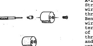
A-14584-A H/L WIRE PLUG Strip insulation from wire and insert bare wire through eyelet in terminal. Bend wire back to parallel wire. Insert wire and terminal into larger end of plug. Insert screw through small hole in plug and thread into terminal until tight.
